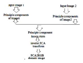
Fig. 3.4 Structure chart of PCA Based Image Picture
